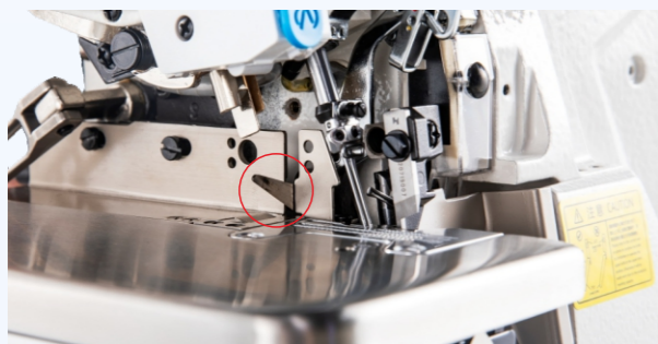
Auto-trimmer, say goodbye to long thread tails save more time, effort and thread.
